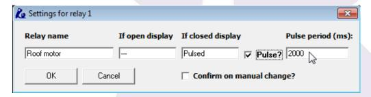
You can name the relay and what should appear when it's closed and open. You can also define it to be a "pulsed" relay, as appropriate in the roof motor configuration. The pulse period, you surely guessed it, is the approximate duration of the pulse in milliseconds.
