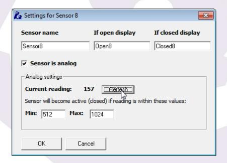
...like shown in the image. Clicking "refresh" will update the current reading. The goal is determining the range of values where we can consider the object is in its place. In our example, the mount is parked, so we could:
