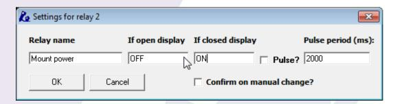
... please continue to do the same for the CCD power and observatory lights – don't forget the lights will be off if the relay is closed!
