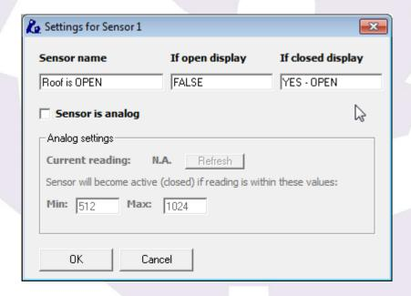
For the roof (roll off roof) we suggest using two switches, one for signalling "open" and another one to signal "closed", this way we will notice should the roof stop mid-way.
