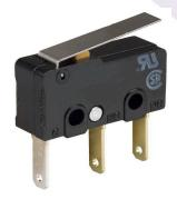
This kind of switches (there are many versions) are quite nice as they provide some play and thus don't require exact roof positioning. If you were using this model, connect the wires to the common (C) and normally open (NO) contacts.
