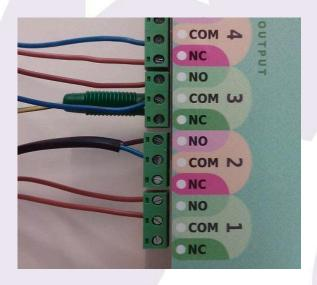
Image taken just after wiring the observatory lights – note the COM-NC connection, as opposed to the rest of the relays.
