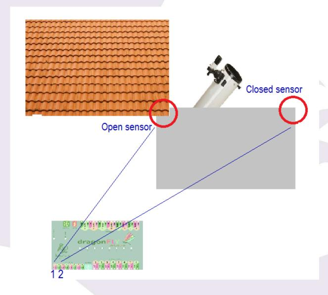
With the software, confirm that the sensor 1 becomes active when the roof is open (inactive otherwise), and likewise for sensor 2 and the roof closed.
