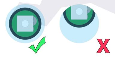
3. **Cables must not be visible through the window**. Sometimes when closing the Cloudwatcher you might notice that the lid cables are covering the "view" of the light sensor. Make sure that the cables get out of the way when closing the lid.
