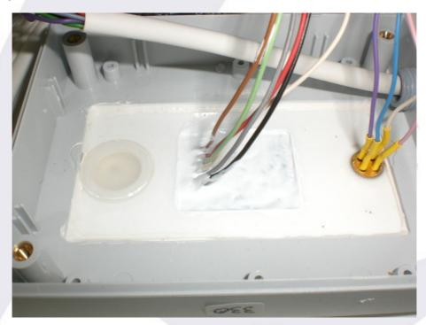
Press firmly from the outside to free the sensor (it's glued to the cover)
